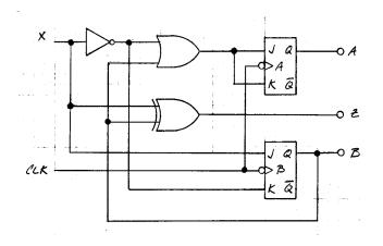
1. Construct a timing diagram for the input sequence:
